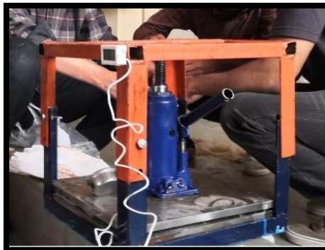
Figure 2. Self-Made compression moulding set-up
