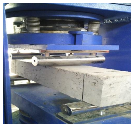
Figure.6. Setup for Flexure Strength Test
