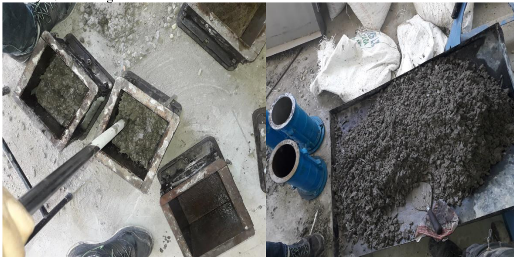
Figure.4. Casting of Specimens
